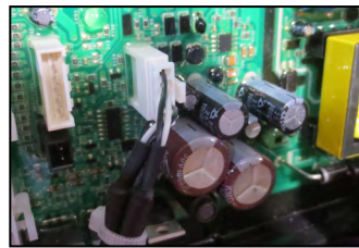
Figure 35 - Cable Wired to Board
